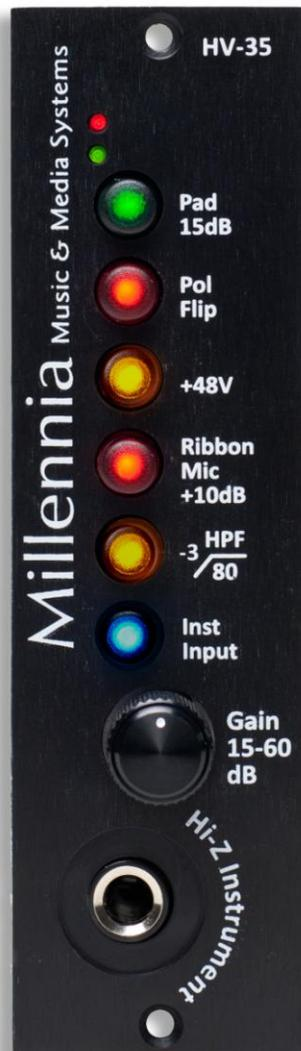
**+48V** turns the phantom power supply on.
