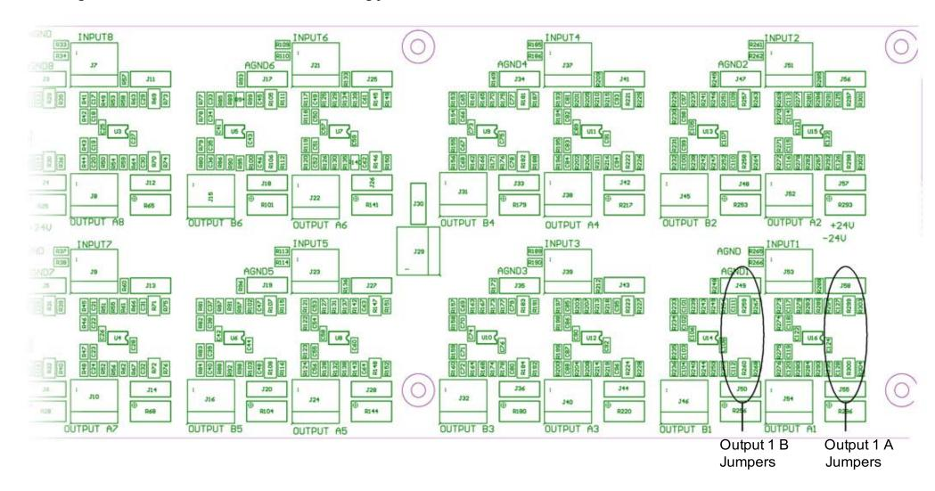
Move pair of jumpers to the left (default) for no output attenuation, to the right for 13.5 dB attenuation Each channel output is individually adjustable
