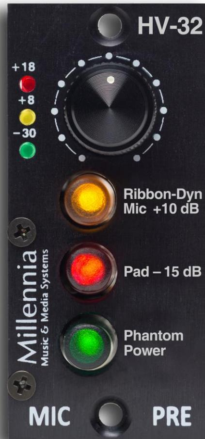
**Gain** is a continuously variable gain control. It has a high gain jump near full clockwise for low level signals.
